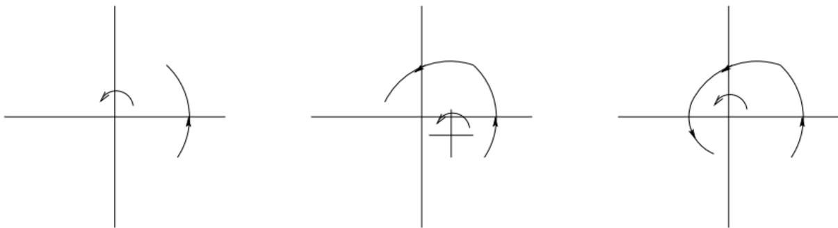
A sequence of changes on the sail orientation implies a sequence of rotations around different equilibrium points on the centre projection, which can result of an unbounded growth.
