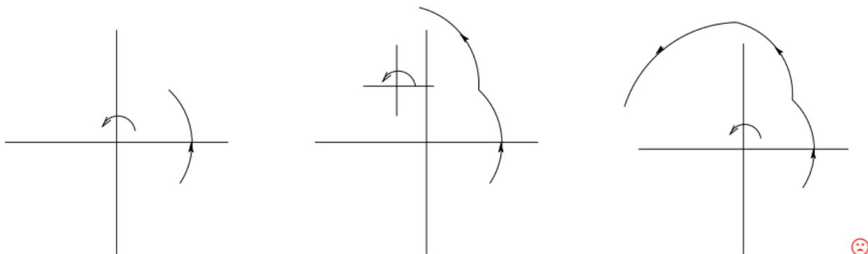
A sequence of changes on the sail orientation implies a sequence of rotations around different equilibrium points on the centre projection, which can result of an unbounded growth.
